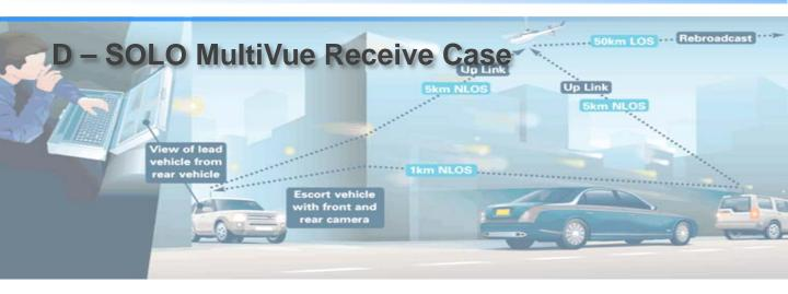
The MultiVue is a briefcase receiver package for teambased tactical video surveillance operations. It will simultaneously decode and display four separate digital video channels, allowing its operator to observe and coordinate the activities of four separate team members operating in different locations. Typical applications include first responder and emergency teams. Equipped with dual diversity antenna inputs, the MultiVue ensures excellent video reception quality.
